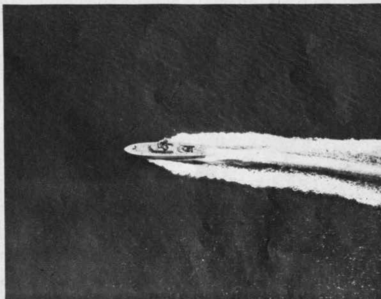
High-speed 85-footer has clean lines, rounded stern. Note the three round gun positions—two atop the low cabin each of which carry twin machine guns, and one in the deck-well equipped with 20-mm. cannon.
